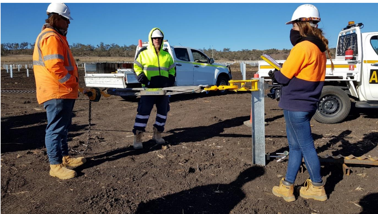
In-service pile testing – Lateral load test
