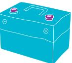
Wet cell batteries use a liquid electrolyte, commonly lead-acid or nickel-cadmium cells.
